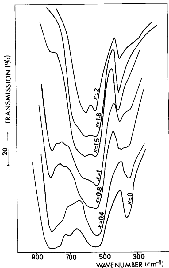
Figure 10 Evolution with composition x of the IR spectrum of iron chromium aluminate spinels in the discontinuity region (temperature 900°C).
